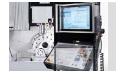
E. Control Panel Ergonomic operation panel with adjustable angle.
