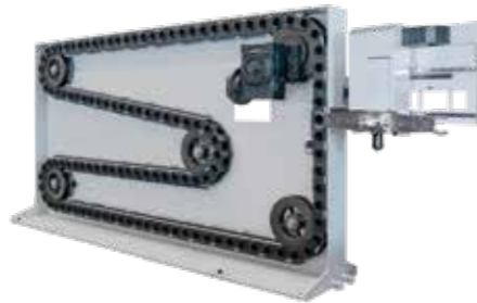
B: Automatic vertical and horizontal ATC system
