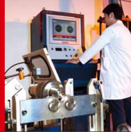
• Spindle, gear box, and spindle motor balance test.
