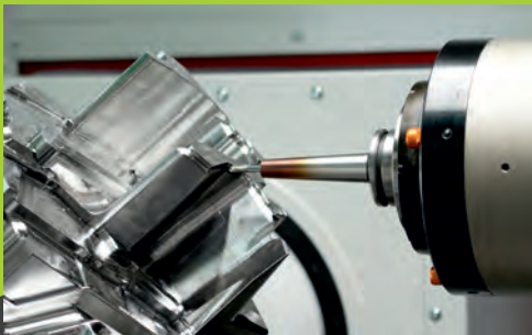
Horizontal Machining Centre with Angular capacity and Deep Hole Drilling
